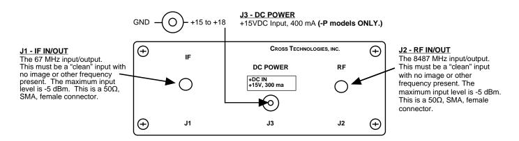
FIGURE 2.3 Model 2009-8487P Rear Panel Inputs and Outputs
