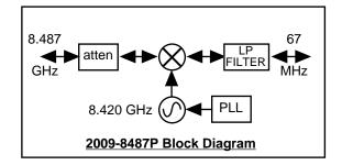
FIGURE 1.2 Block Diagram
