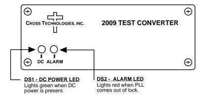
FIGURE 2.2 Model 2009-8487P Front Panel Indicators
