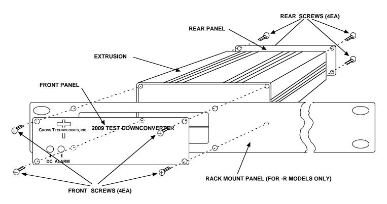
FIGURE 2.1 Model 2009-8487P Assembly (-R option shown)
