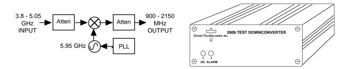
FIGURE 1.1 Model 2009-38 Block Diagram and Chassis
