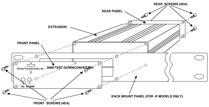
FIGURE 2.1 Model 2009-138 Assembly (-R option shown)
