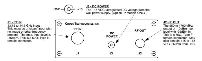
FIGURE 2.3 Model 2009-138 Rear Panel Inputs and Outputs
