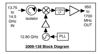
FIGURE 1.2 Block Diagram
