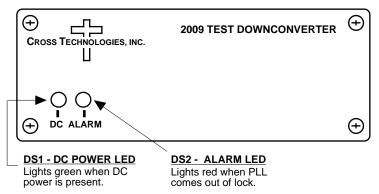
FIGURE 2.2 Model 2009-138 Front Panel Indicators
