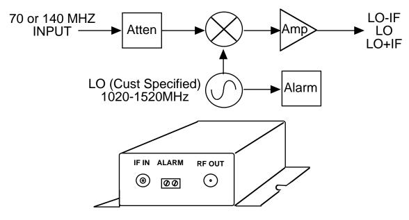
FIGURE 1.1 2006-04 Upconverter Block Diagram and Chassis
