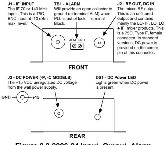
Figure 2.3 2006-04 Input, Output, Alarm Power LED, External DC In (-P, -C Options)
