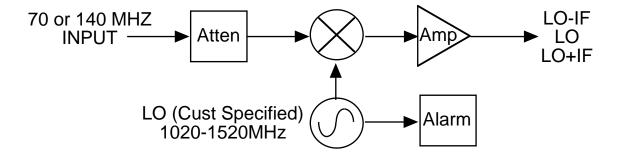
FIGURE 3.1 Block Diagram
