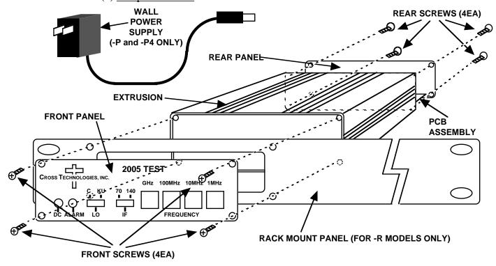
FIGURE 2.3 2005 Assembly Drawing
