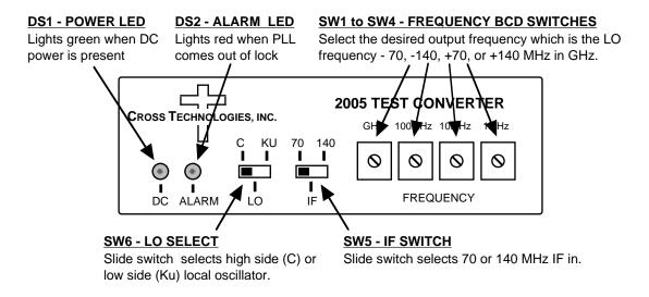
FIGURE 2.1 2005-10P Front Panel Controls and Indicators
