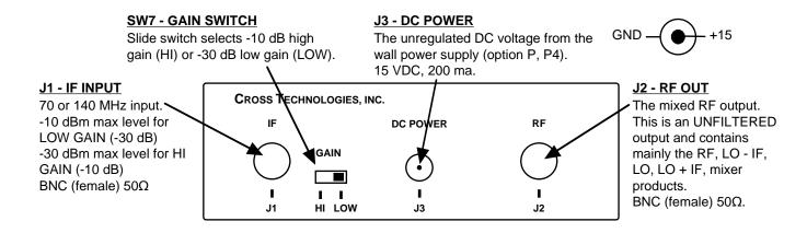
FIGURE 2.2 2005-10P Rear Panel Inputs and Outputs
