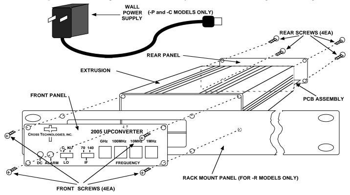
FIGURE 2.1 2005 Assembly Drawing
