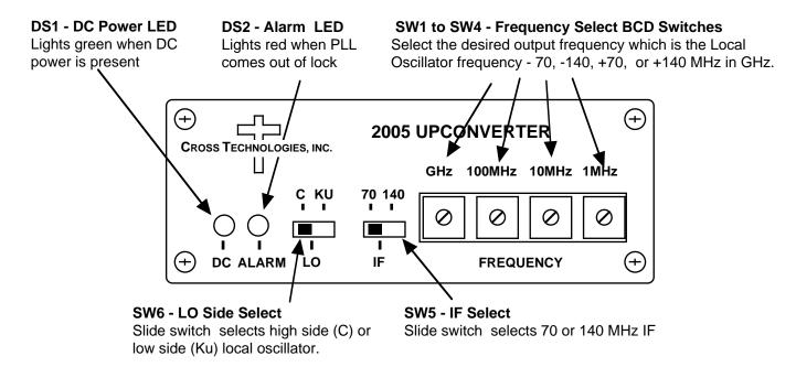
FIGURE 2.2 2005 Front Panel Controls and Indicators
