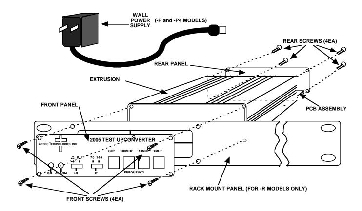
FIGURE 2.3 2005 Assembly Drawing
