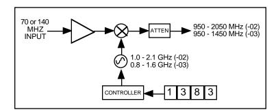
FIGURE 1.2 Block Diagram
