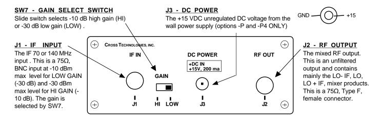
FIGURE 2.2 Rear Panel Inputs, Outputs, and Controls
