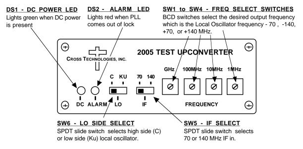
FIGURE 2.1 Front Panel Controls and Indicators
