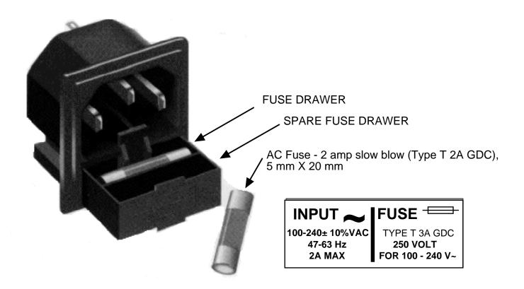
FIGURE 2.4 Fuse Location and Spare Fuse
