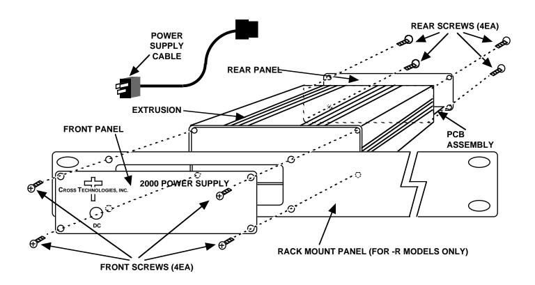
FIGURE 2.1 Mechanical Assembly (Rack Mounting)
