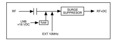
FIGURE 1.2 Block Diagram
