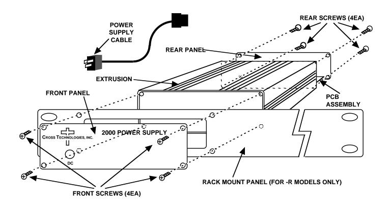
FIGURE 2.1 Mechanical Assembly (Rack Mounting)
