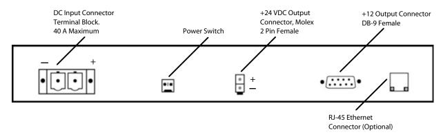
FIGURE 2.3 Side Panel Connections
