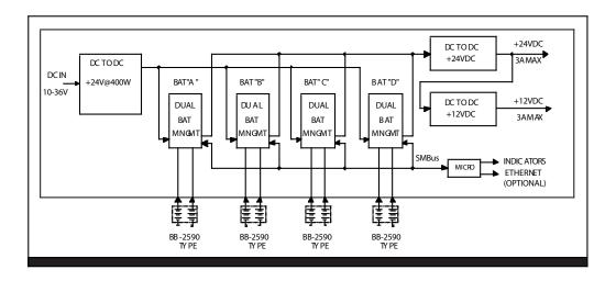
FIGURE 1.2 2000-16-3624 Power Supply/Battery Charger Block Diagram
