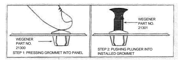
FIGURE 2.1 INSTALLING FRONT PANEL
