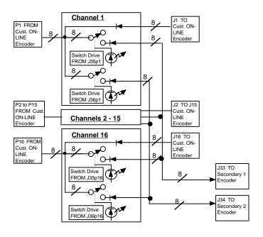
Figure 1.2 Model 162 Cue Switch Block Diagram
