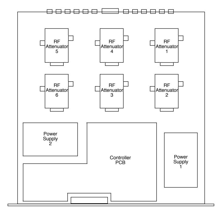
FIGURE 2.0 1586-06 Mechanical Assembly
