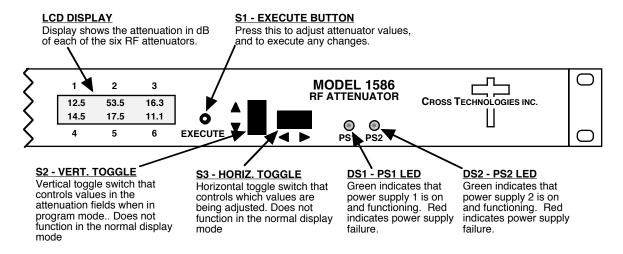
FIGURE 2.2 1586-06 Front Panel Controls and Indicators
