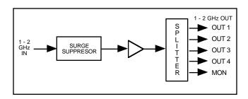
FIGURE 1.2 MODEL 1584-45S Block Diagram (Each Splitter)
