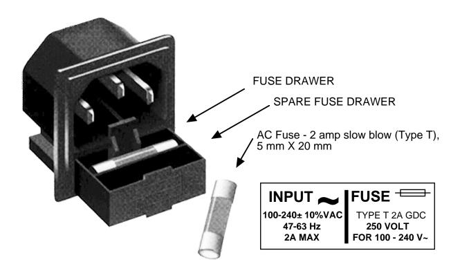
FIGURE 2.4 FUSE LOCATION AND SPARE FUSE
