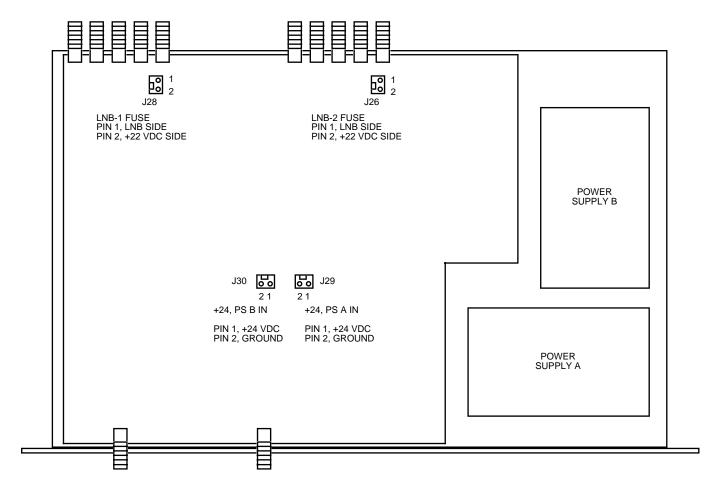
FIGURE 2.1 1584-25 MECHANICAL ASSEMBLY
