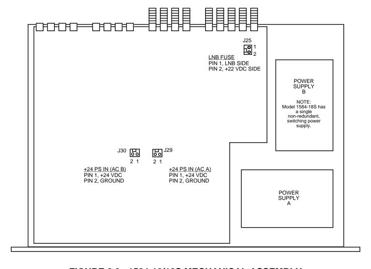
FIGURE 2.0 1584-18/18S MECHANICAL ASSEMBLY
