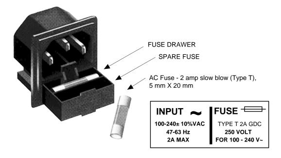
FIGURE 2.6 FUSE LOCATION AND SPARE FUSE
