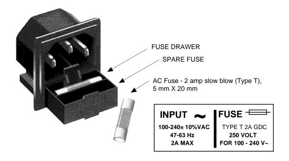
FIGURE 2.6 FUSE LOCATION AND SPARE FUSE
