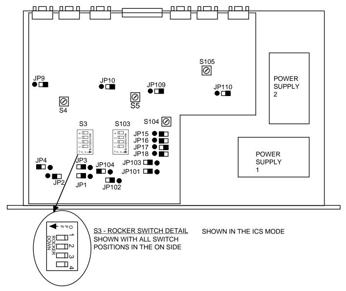
FIGURE 2.3 1582-725 PCB Settings Parts Locations
