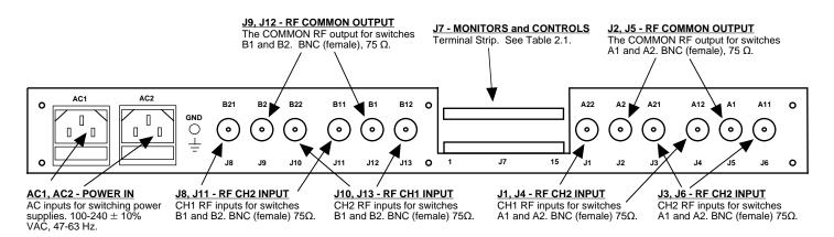
TABLE 2.0 Rear Panel Input/Output Connectors Pinout
