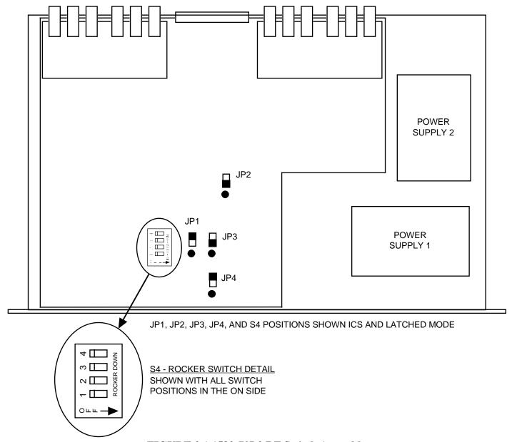
FIGURE 2.1 1582-70L2 RF Switch Assembly
