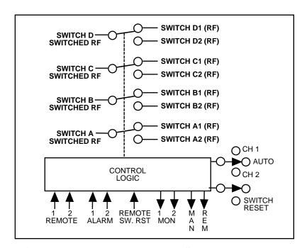
FIGURE 1.2 Model 1582-70L2 RF Switch Block Diagrams
