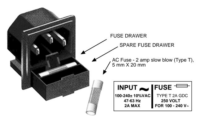
**FIGURE 2.4 Fuse and Spare Fuse Locations**
