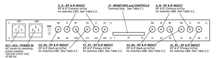
FIGURE 2.2 1582-70L2 RF Switch Rear Panel Inputs/Outputs
