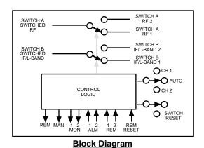
FIGURE 1.2 Model 1582-652 RF Switch Block Diagrams
