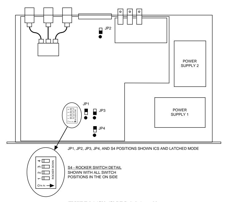
FIGURE 2.1 1582-652 RF Switch Assembly
