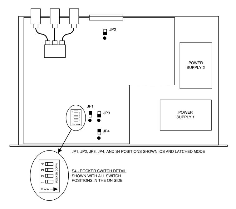
FIGURE 2.1 1582-650 RF Switch Assembly
