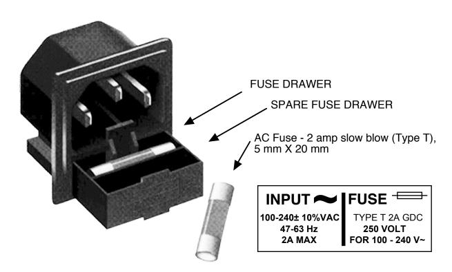
**FIGURE 2.4 Fuse and Spare Fuse Locations**
