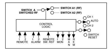
FIGURE 1.2 Model 1582-650 RF Switch Block Diagrams
