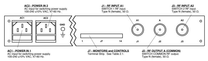
FIGURE 2.2 1582-650 RF Switch Rear Panel Inputs/Outputs
