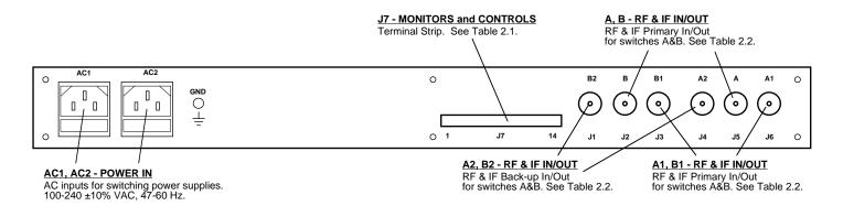
FIGURE 2.2 1582-22L RF Switch Rear Panel Inputs/Outputs
