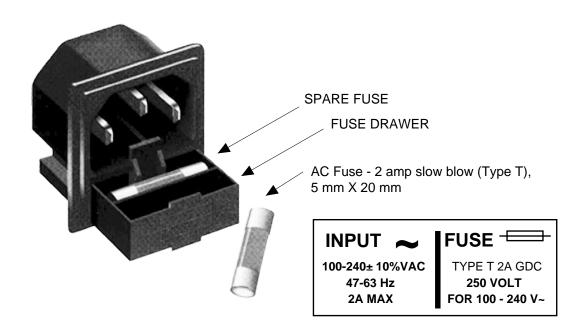
FIGURE 2.4 Fuse and Spare Fuse Locations
