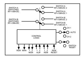
FIGURE 1.2 Model 1582-22L RF Switch Block Diagrams
