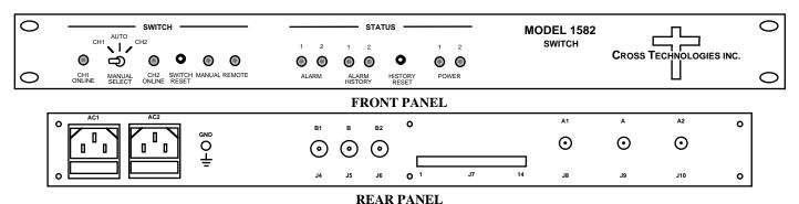
FIGURE 1.1 Model 1582-152 Front and Rear Panels
