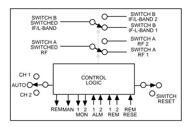
FIGURE 1.2 Model 1582-152 RF Switch Block Diagrams
