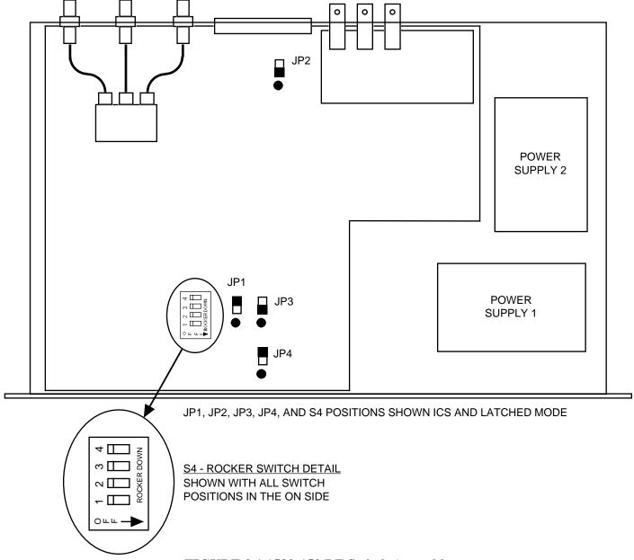
FIGURE 2.1 1582-152 RF Switch Assembly
