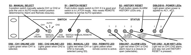
FIGURE 2.3 1582-152 Front Panel Controls and Indicators
