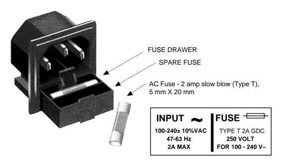
**FIGURE 2.4 Fuse and Spare Fuse Locations**
