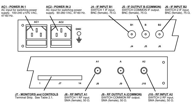
FIGURE 2.2 1582-152 RF Switch Rear Panel Inputs/Outputs
