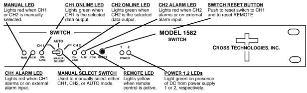
FIGURE 2.2 1582-13 Front Panel Controls and Indicators
