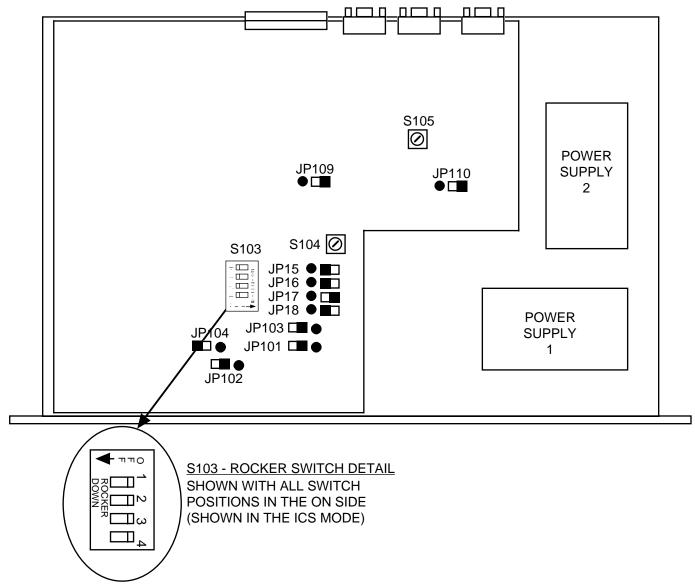
FIGURE 2.3 1582-13 PCB Settings Parts Locations
