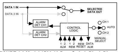
FIGURE 1.2 Model 1582-13 Data Switch Block Diagram
