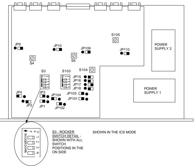
Figure 2.3 PCB SETTINGS PARTS LOCATIONS
