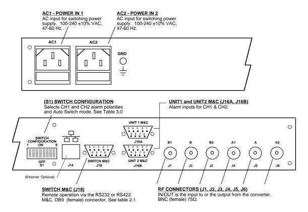
FIGURE 2.2 1582-122L Switch Rear Panel Inputs/Outputs
