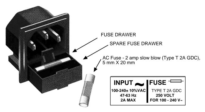
FIGURE 2.4 Fuse Location and Spare Fuse
