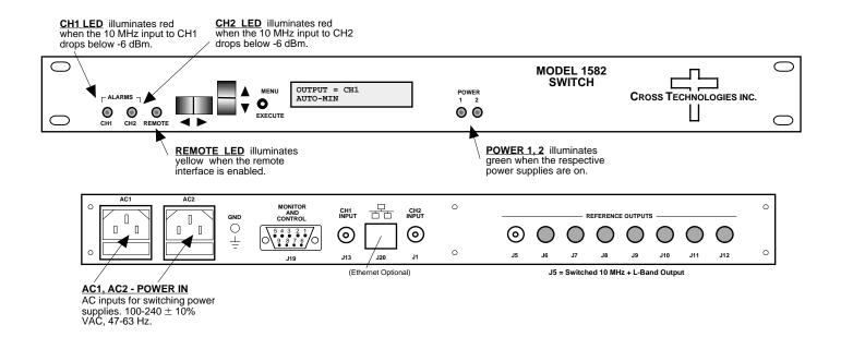
FIGURE 2.3 1582-1001LB Front AND REAR Panel Controls and Indicators
