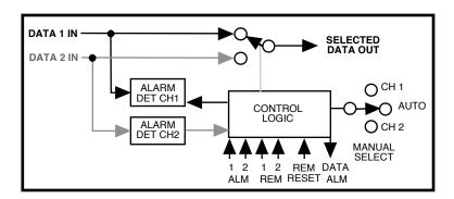
FIGURE 1.2 Model 1582-04 Data Switch Block Diagram (Each Switch)
