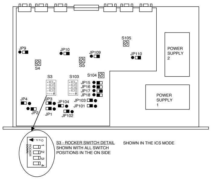
FIGURE 2.3 1582-04 PCB Settings Parts Locations
