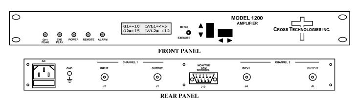
FIGURE 1.1 Front and Rear Panels
