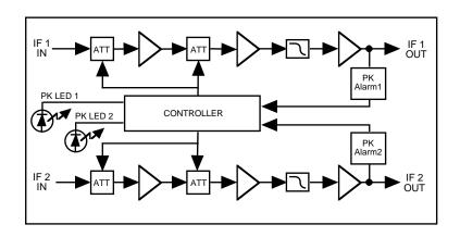
FIGURE 1.2 Block Diagram
