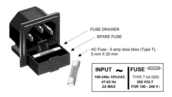
FIGURE 2.4 Fuse Location and Spare Fuse
