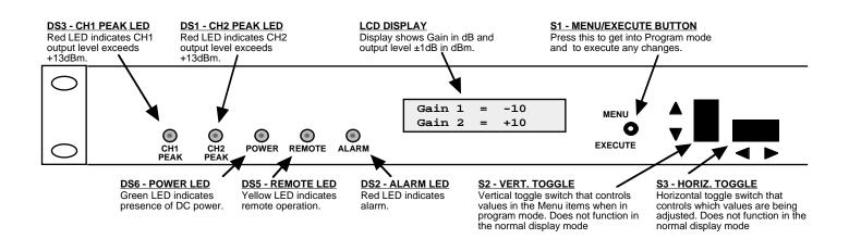
FIGURE 2.3 Front Panel Controls and Indicators
