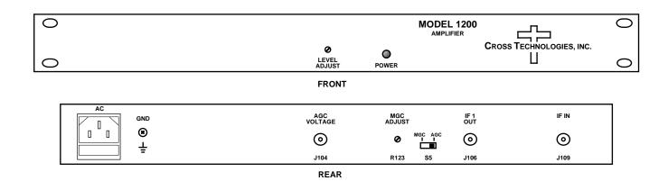
FIGURE 1.1 Model 1200-75 Front and Rear Panels
