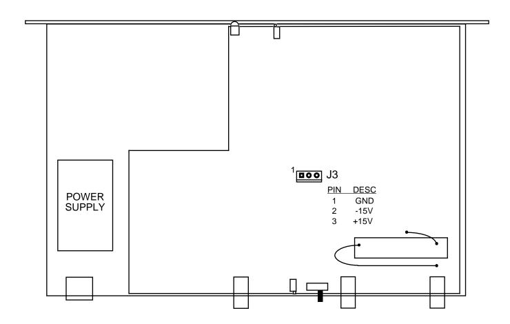
FIGURE 2.1 1200-75 Mechanical Assembly
