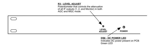
FIGURE 2.3 1200-75 Front Panel Controls and Indicators
