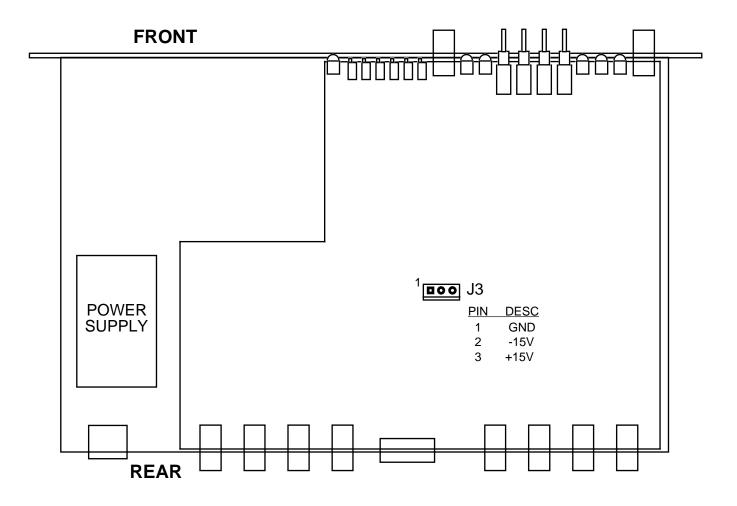
FIGURE 2.1 1200-05 Mechanical Assembly
